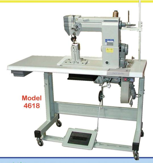
The ARTISAN® model 4618 post bed machines is an extremely high quality lockstitch single needle, needle feed, driven roller presser foot and roller feed sewing machine with a semi-automatic lubrication system. The machine is designed for stitching very light to medium heavy leathers, boot tops, shoes and upholstery fabrics where quality stitch formation is of the utmost importance.
