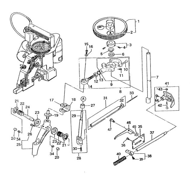
(3) NEEDLE BAR, PRESSER BAR AND DRIVING PARTS
