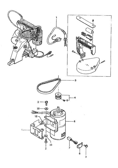
(6)MOTOR, PARTS (For totally Enclosed Type Motor)
