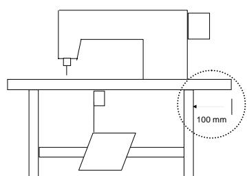
b). Mounting HVP-70 under the working table
