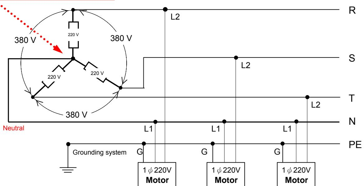
(3). The load balance when use a 1Φ / 220 V motor used on a 3 Φ / 220 V power source.
