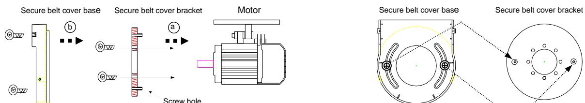
C). After install base, mount with the motor pulley and secure it.
