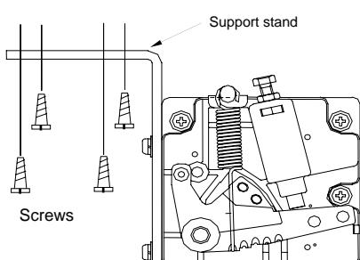
b). Keep rod in vertical, secure the unit under the table
