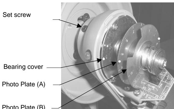
Needle up position : Rotate the machine pulley to reach mechanical needle up position and turn the photo plate (A) until its red mark is aligned with the red mark on the bearing cover plate.
